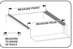
A. Measure distance between inside rails at selected front location. Measure distance between inside rails at selected rear location. See Diagram. Record both of these measurements for step C.
