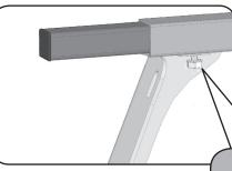
A. Finish tightening all cross bar hex head bolts by turning bolt completely in until serrations on flange are seated tight. Doing this means the bolt will push up on the wall of the cross bar hidden inside upright tube.
