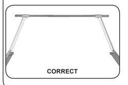
D. CORRECT. Cross bar centered without binding between uprights- bar is level and ready for next step.
