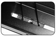
C. **Pull up on cord** until you can see and feel that all plates and clamp are held up against bottom of stake pocket and rail as shown. Continue pulling up tight on cord for next step.
