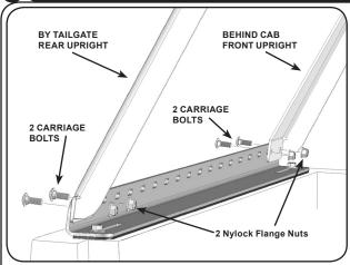
A. Set assembled front cross bar/uprights up in between front rails. Align both uprights as shown and bolt with 2 carriage bolts and nylock flange nuts. NOTE: Uprights should fit nicely in between rails. If they don't, make needed adjustments before bolting tight, then turn nuts fully tight now. Repeat procedure for rear up right assembly.
