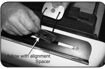
B. Continue dropping each alignment plate one at time through slot and into stake pocket. Hold cord firmly, jiggle it around and up and down as needed until clamp and plates align with stake pocket for next step.
