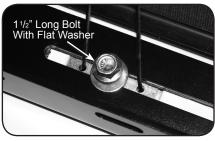
D. Place flat washer over hole and thread a hex head bolt into threaded clamp inside stake pocket. Turn until finger tight. **Ensure that alignment plates are aligned with stake pocket.** Then remove cord. Repeat A through D for all remaining stake pockets.
