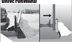
The blade is guided by a push frame that allows it to slide up and down with the grade of the terrain.
