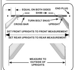
C. Slide front cross bar (the bar without reflective decal) in uprights. Space bottom of uprights to match front measurement taken earlier between rails. Center cross bar. Turn set bolt in temporarily snug enough to prevent cross bar slippage. Tap end plug into each end of cross bar.
