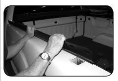
B. Carefully place rail on top of box rail with slotted holes centered across stake pockets.
