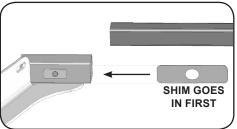
B. Lay uprights and cross bar on floor as shown. Slide shim inside tube of each upright until both holes line up.
