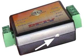
With the throttle at idle, start the engine and turn on brake switch. Then, using a small flat bladed screwdriver, turn the small adjusting screw in the DFIV Module counterclockwise or clockwise until the test light JUST turns on.
